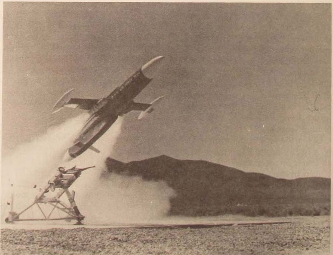
The Tactical Expendable Drone System (TEDS) is a decoy and jamming platform for use with strike aircraft.
