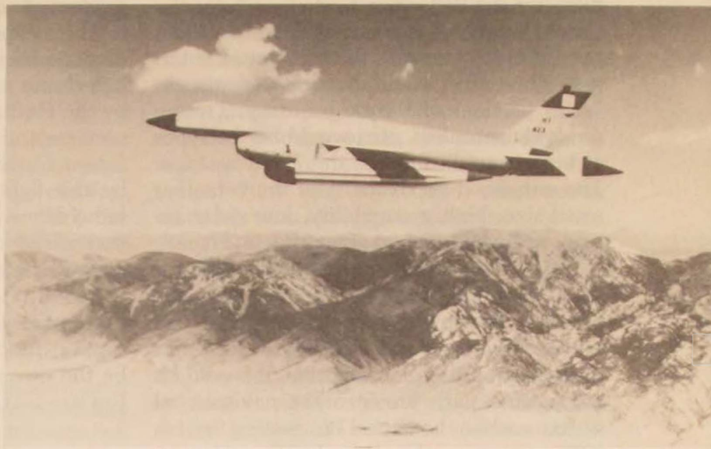
Combat Angel, an electronic warfare support remotely piloted vehicle, carries chaff pods and nose-jamming transmitters. It is flown by a Tactical Air Command drone squadron.
